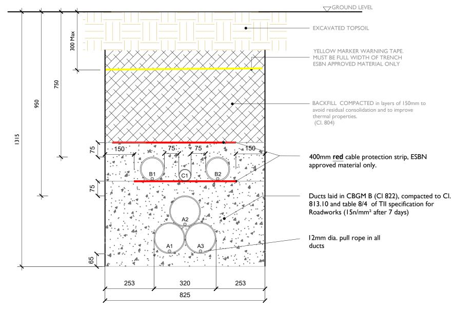
A = 160mm: Outer Diameter HDPE ESB Approved Duct, SDR=21 (Power) [ESB Code: 9317552]
